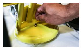
5. Remove the pin, place the handle in the low position and re-pin.
