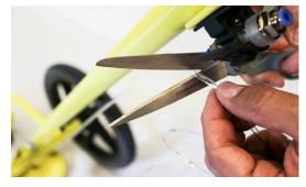
6. Snap the tubing into the tubing clips along the handle keeping the slack on the lower side.
